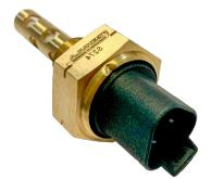
Featuring an integrated Deutsch DT04-3P connector the **\$274** is a capacitance type oil level switch for use in mineral oils including engine, transmission and hydraulic oils. It is an active device designed to give an alarm signal if oil falls below, or rises above, a preset level. It can also be specified with a delay to eliminate false alarms due to turbulence.
