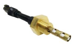
The **S288** is an active device designed to give an alarm signal if liquid falls below, or rises above, a preset level. It can be specified with a delay to eliminate false alarms due to turbulence. A flying lead enables customers to specify a suitable connector of their choice.
