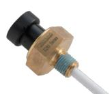
The **S285** is an active device designed to give an alarm signal if liquid falls below or rise above a preset level. It can be specified with a delay to eliminate false alarms due toturbance. Containing a factory programmable microprocessor, the switch offers sink to ground a reduced risk of damage and a wide range of customer specifiable options make it suitable for most applications.
