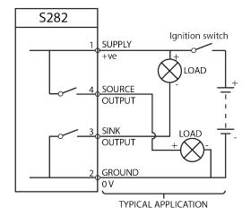
NOTE: IF SINK ONLY OUTPUT IS REQUIRED THEN PIN 4 IS NOT USED.
