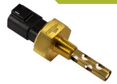
The **\$284** is an active device designed to give an alarm signal if liquid falls below, or rises above, a preset level. It can be specified with a delay to eliminate false alarms due to turbulence.
