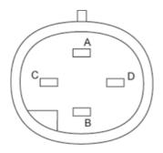
NOTE: Pin B on configuration 1, 2 and 3 is used for 4-20mA loop. On configuration 4, 5, and 6 the connection is used for Low Level Alarm.
