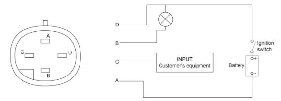
Note: Pin B has the option to be a communications port rather than an alarm if factory configured at the time of ordering.
