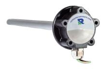
T he **T/LL350** series is a range of highly advanced sensors for continuously measuring the contents of a tank. The unique feature of the T/LL350 is that it auto compensates when a liquid with a different d electric constant is used. For example, if it is used in a tank of conventional diesel, then the user c an refill with bio-diesel and the sensor will correct the output level automatically.
