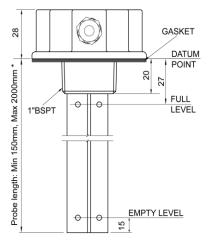
\* Up to 1000mm in mobile applications or up to 2000mm in static applications.
