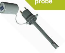
The **Model OP/02** tank overfill prevention probe is designed for use in static bulk storage fuel tanks and operates by passing a signal back to the fuel delivery system when the fuel reaches the maximum filling level.
