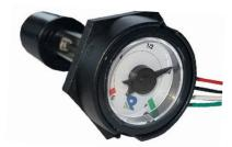
The **G/LL65** vertical spiral gauge is a mechanically operated liquid level gauge with a local display and two electrical outputs. Suitable for connection to a typical controller or remote level indicator the outputs are; a variable resistance proportionate to the liquid level and a volt-free switch to trigger an alarm when the liquid reaches a prescribed level.
