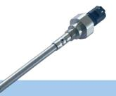
The T/LL415 Liquid Level Sensor is an advanced capacitive level sensor that continuously monitors liquid level and temperature and broadcasts this via a CAN J1939 output protocol.
