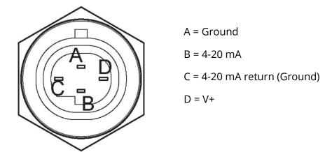
Matting Connector: Rochester Sensors C/K1 (4-way Delphi Packard Metri – Pack 150 series). To fit 8.0-1.0mm<sup>2</sup> conductor, Ø1.6-2.15 mm sleeve.
