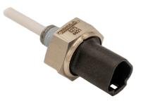
Featuring an integrated Deutsch DT04-3P connector the **S273** is a capacitance type liquid level switch for use in water-based liquids including engine and battery coolants. It is an active device designed to give an alarm signal if liquid falls below, or rises above, a preset level. It can also be specified with a delay to eliminate false alarms due to turbulence.
