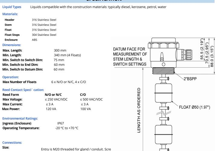
Entry is M20 threaded for gland / conduit. Scre Terminals for Ø2mm / 3 mm<sup>2</sup> conductors.
